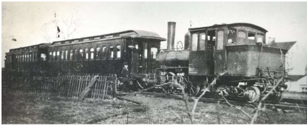
Former New York City Elevated Railway "Forney" type locomotive, renumbered "1," and NY City Elevated Ry. coaches being used on the Washington, Frederick & Gettysburg Railway.
