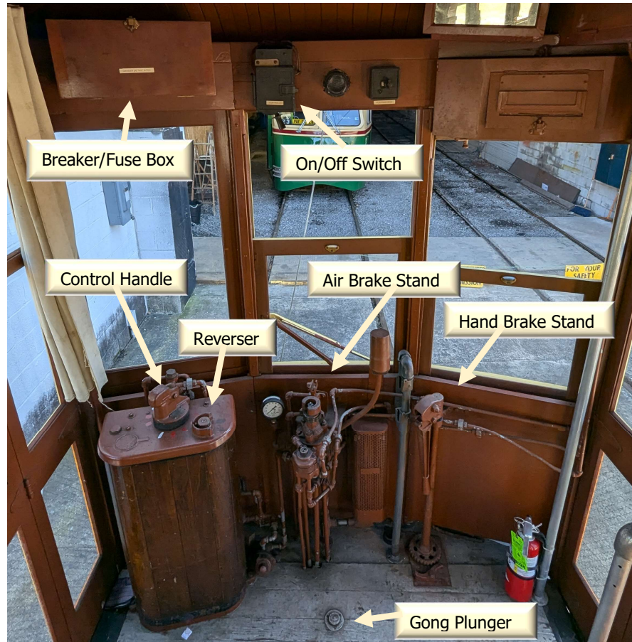
A parked trolley at the Rockhill Trolley Museum demonstrates common locations of things referenced in this section and the next. Note that the actual handles of the control stand and brake stand have been removed, as was normal whenever parking a trolley in order to avoid unauthorized movement.
